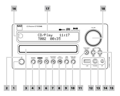
1 **POWER:** Press this button to switch ON the C 715. The Standby LED indicator will turn from amber to blue and illuminate the Vacuum Fluorescent Display (VFD). Pressing the power button again turns the unit back to standby mode.
